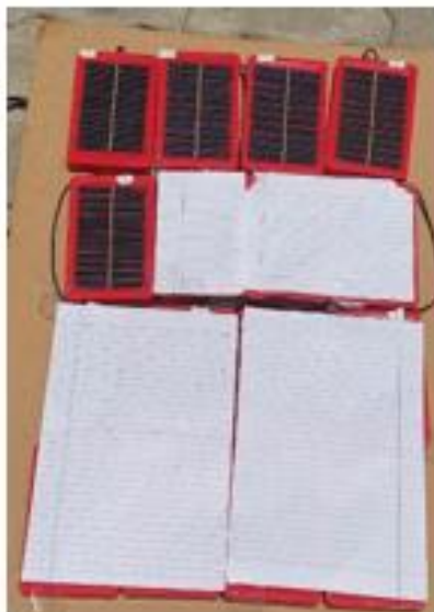
Fig 6.5 LW shading on MS configuration.
