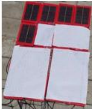
Fig 6.4 LW shading on TCT configuration.
