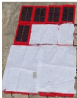
Fig 6.2 LW shading on BL Configuration
