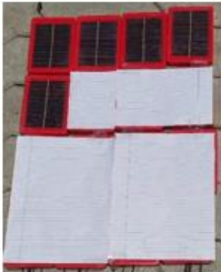
Fig 6.3 LW shading on HC configuration
